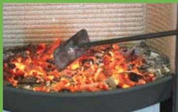
After 5-10 min. the heat will create a draw through the chimney and the door can be closed. After a further 10-20 min. there will be a good layer of embers in the chamber. Use a poker to spread the embers around the bottom and add more fuel.
