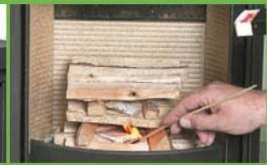
Arrange a pile of dry kindling, approx. 1-2 kg, enough to create a good layer of embers. Light the fire lighters. Leave the stove door ajar.
